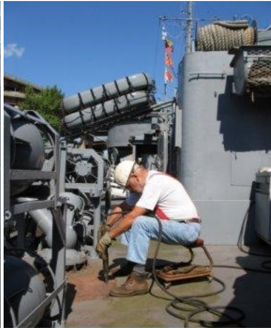
Chris Fedden and his chipping tools work their way forward to continue the never ending job.
