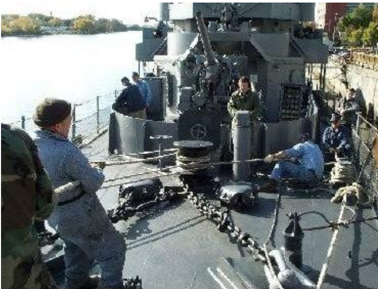
Using the windlass to bring the whaleboat aboard.
