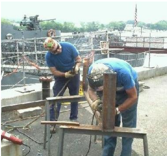
Tanner and Benner fabricating the gangway saddle.
