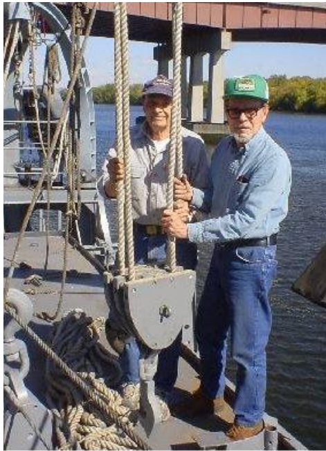
Rocky and Roy rigging the new boat falls.
