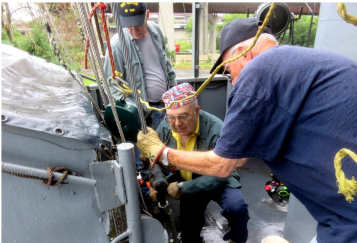
Adjusting the tension on the new shrouds.
