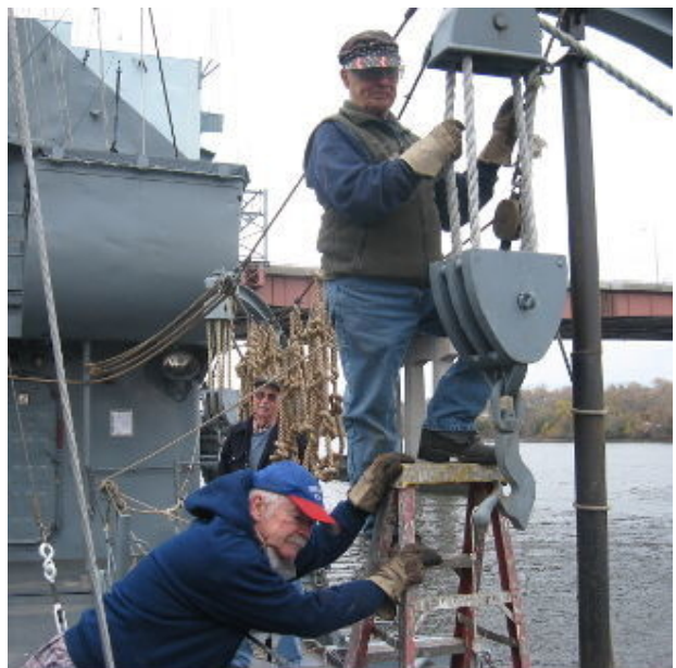
The deck gang breaking down the temporary supports on the aft davit.
