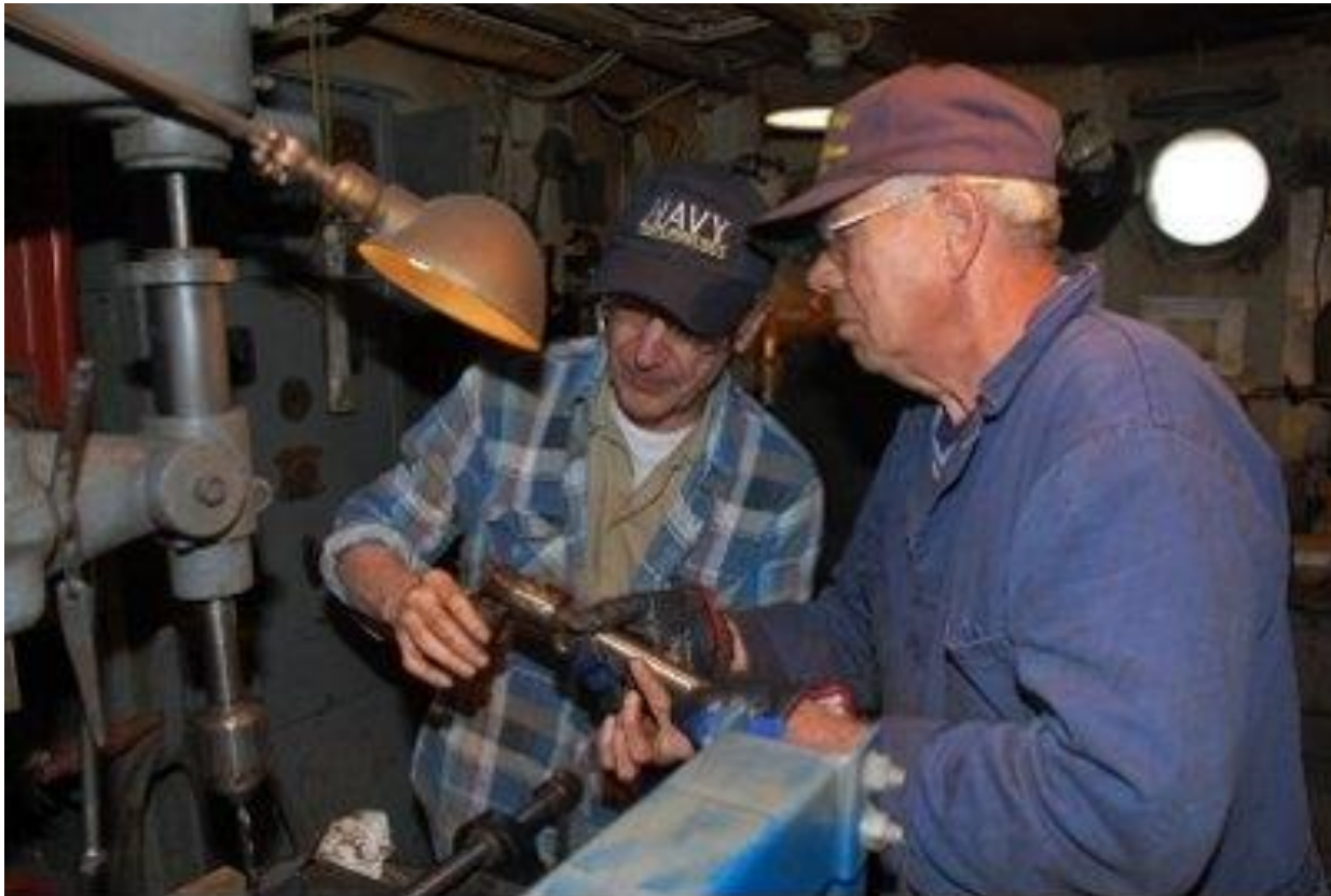
Gary Dieckman and Butch Warrender putting new bearings on the gun 1 gear shafts.
