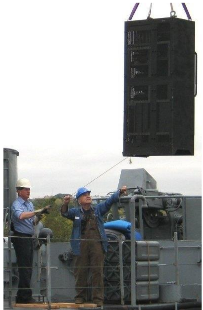
"Battleship" Mike and Doug Tanner reach for the new TBL transmitter as it is hoisted aboard SLATER.
