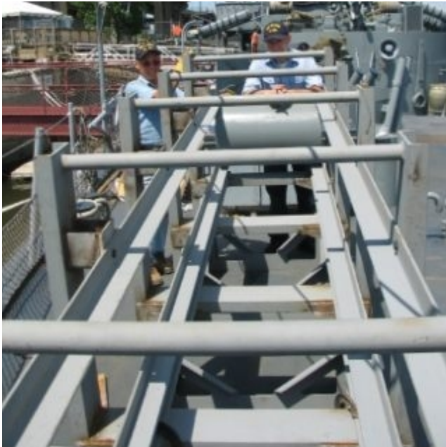
The first depth charge rolls into the new port side fantail rack.
