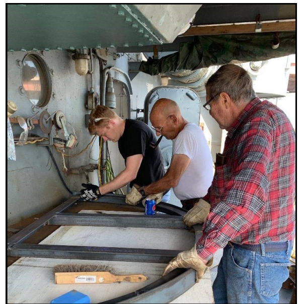
RPI Midshipman Brendan Lutz, Tim Benner, and Danny Statile got the major parts of the SL surface search radar maintenance platform tacked together.
