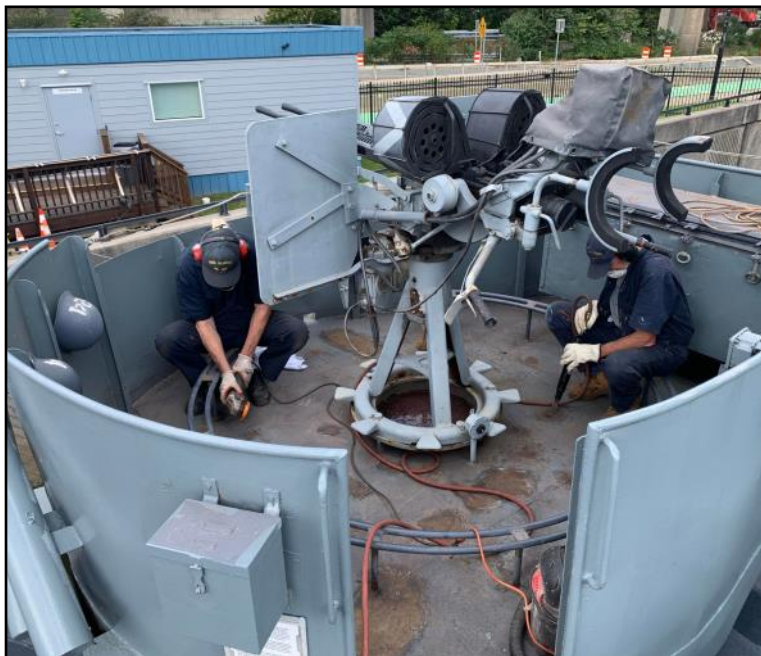
Our two Ronnies chipped out the 20mm gun tubs. You can't needle scale without compressed air.
