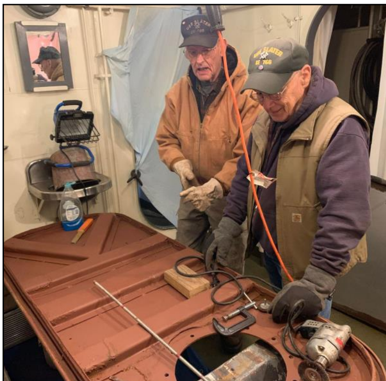
Tim Benner and Super Dave Mardon finished priming the watertight door.
