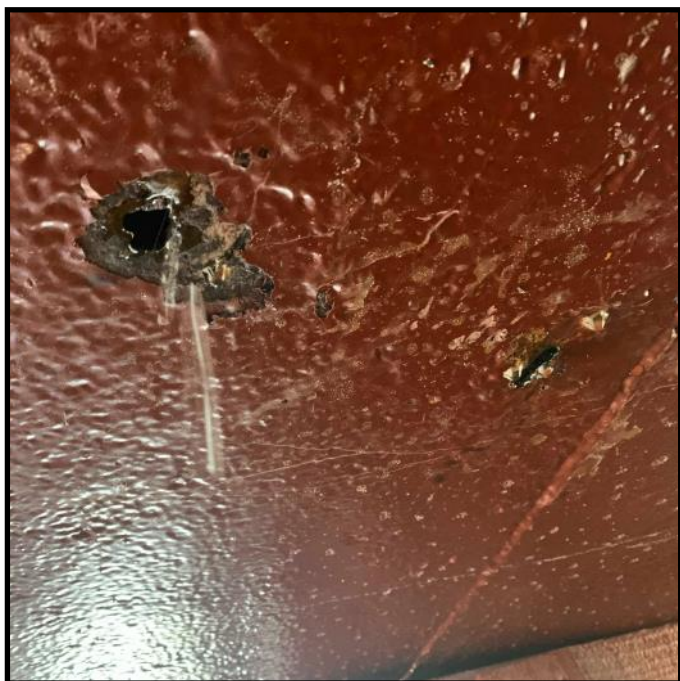
Quarter sized leak in the hull prevented us from returning on Friday.
