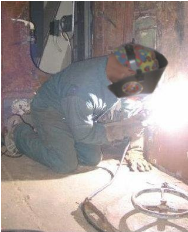
Tim Benner welds in replacement bulkhead in the forward passageway.
