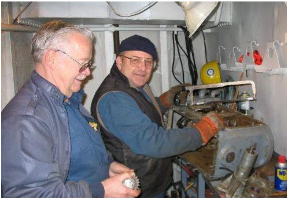
Karl Herchenroder and Gus Negus working on the train gear drive from gun two.
