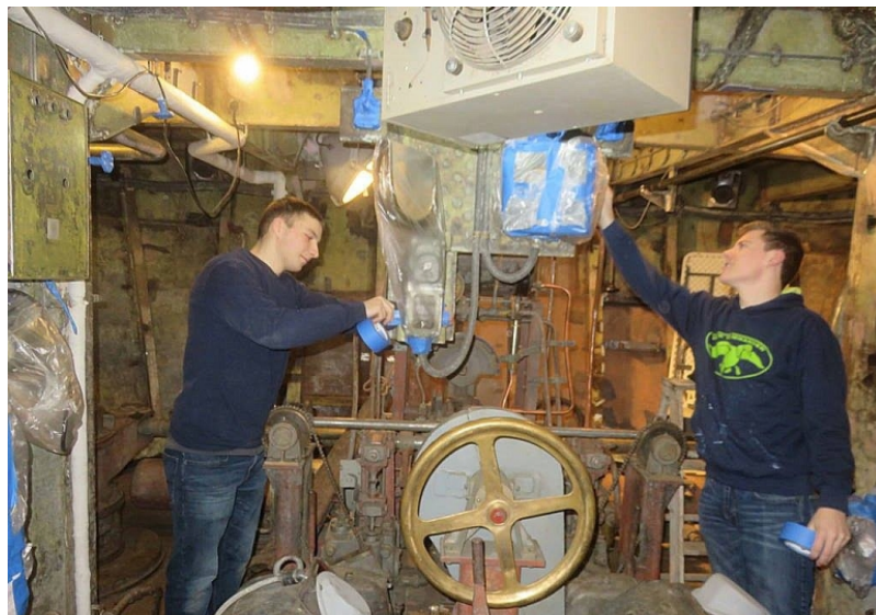
RPI Midshipmen masking the steering gear for painting.
