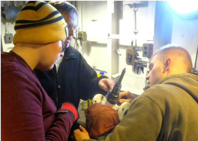
Barry Witte instructing students on valve overhaul. The RPI Midshipmen and NPTU Sailors are gaining practical experience by volunteering on board.
