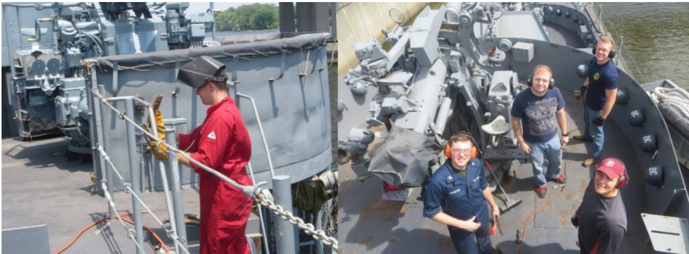
Shipfitters from NPTU replace a ladder handrail and students from NPTU work outside their rate, scaling decks, topside.
