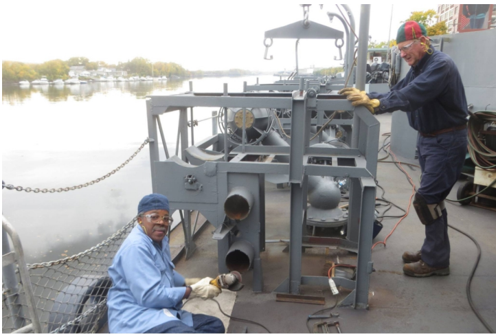
Ralph Griffen and Bob Lally making repairs to the depth charge roller loaders.
