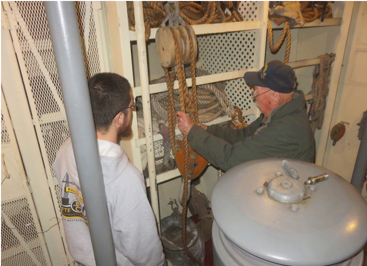
Ken Powers and Boats Haggart rigging a new block and tackle.
