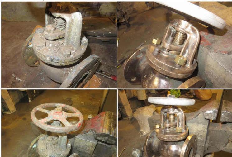
Before and after views of Thomas Scian's valve restoration.
