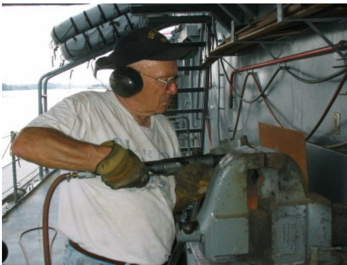
As always, Dave is hard at work! Here, he is chipping paint and rust off a fantail rack part.
