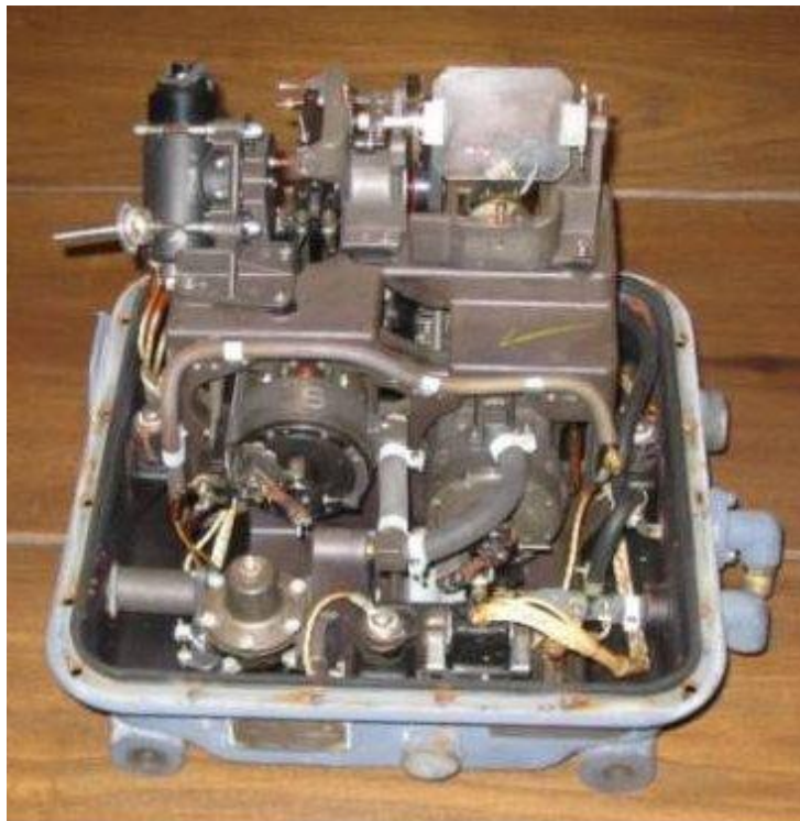
A MK14 gunsight ready for its cover to go back on. It's a secret weapon so don't look too closely at it!
