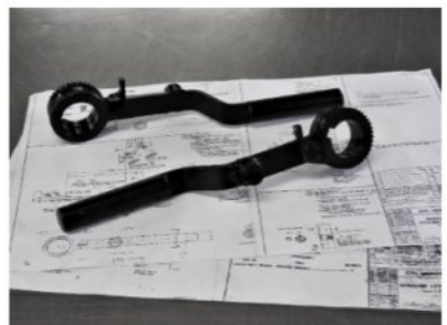
20mm magazine drum loading ratchets fabricated from scratch by George Christophersen.
