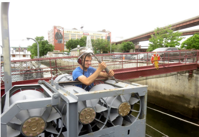
Volunteer Thomas Scian scaling depth charge roller loader number six.
