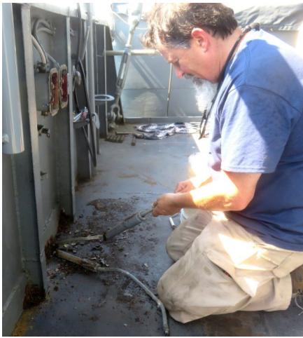
Rewiring the signal lamp, step one. Steve Klauck pulls the old wires. I think these stuffing tubes are shot.
