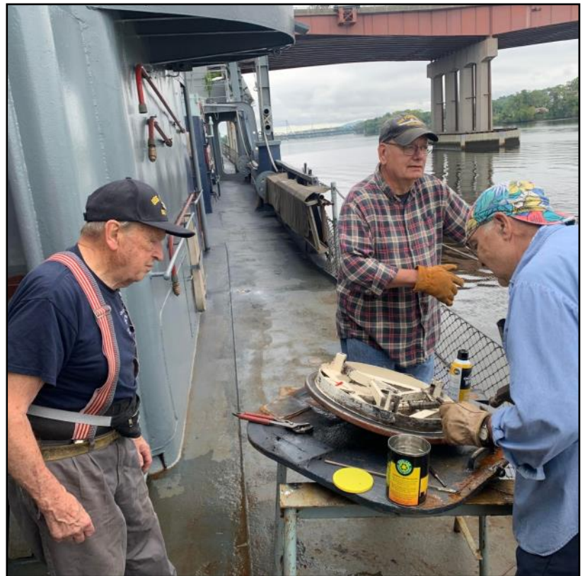
Another day, another scuttle repair job.
