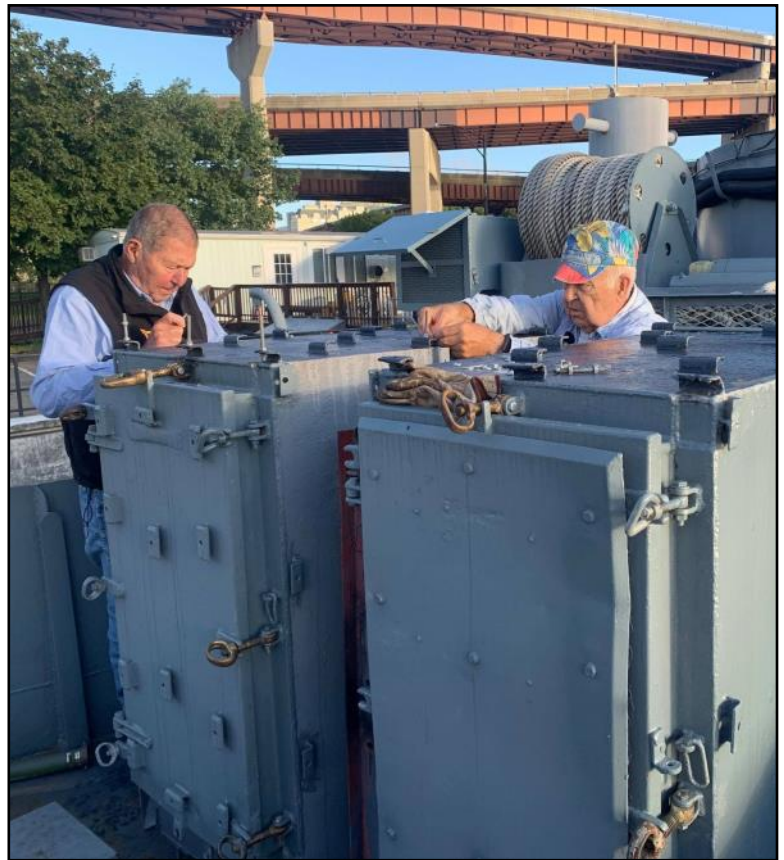
Danny and Doug are fitting the heat shields on the gun 33 ready service lockers.
