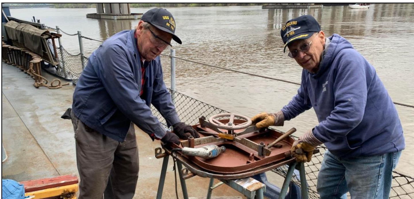
Gene and Dave completing the adjustments to the foc's'cle hatch.
